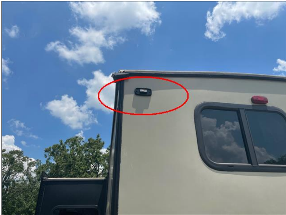
Streetside rear clearance light
