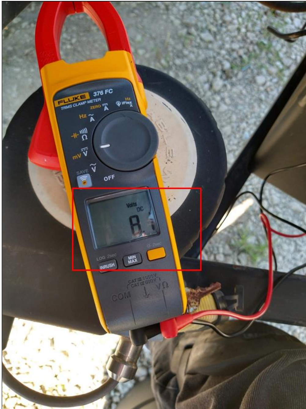
Battery Voltage Test
